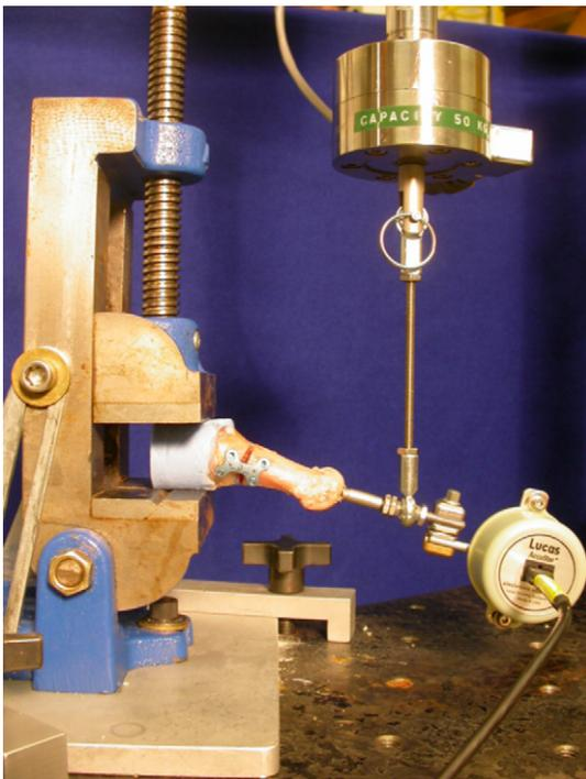
Fig. 2. First metatarsal mounted in testing machine. Load was cyclically applied in plantar-to-dorsal direction while monitoring load, displacement, and angulation.
